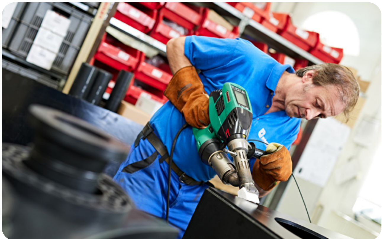
Fig.: Welding of PE panels
