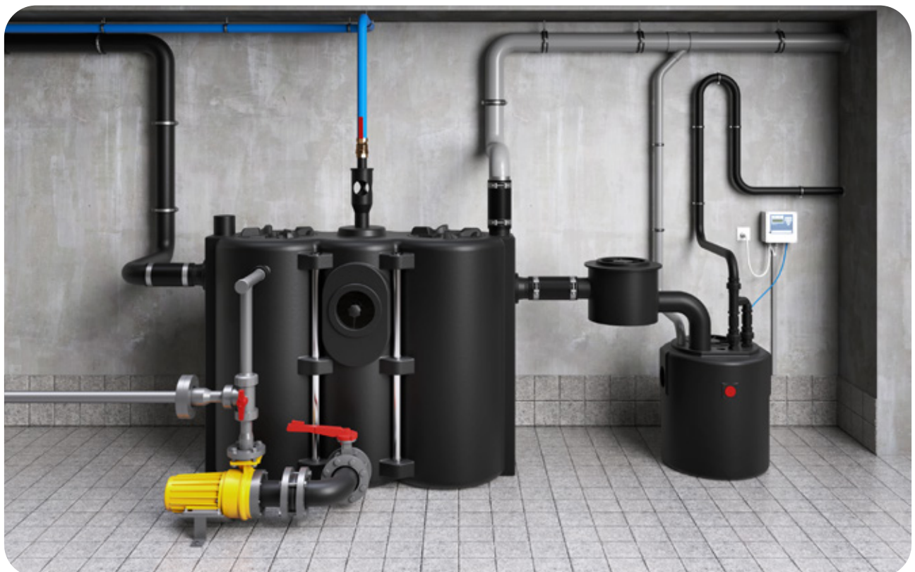
Fig.: Grease separator NS 4 with rinsing and disposal facilities, sampling unit DN 150
